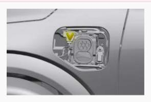
Yellow light indicates that the charging handle is plugged in, and it is in a authentication process.
