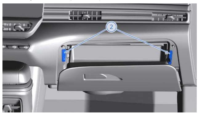
2. Carefully push in the sides of the glove box past the two side clips
