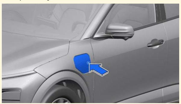
3. Press on the charge port door as shown above to open.
