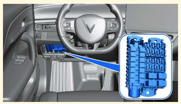
The Instrument Panel fuse box is located in the lower left-hand side of the dashboard.
