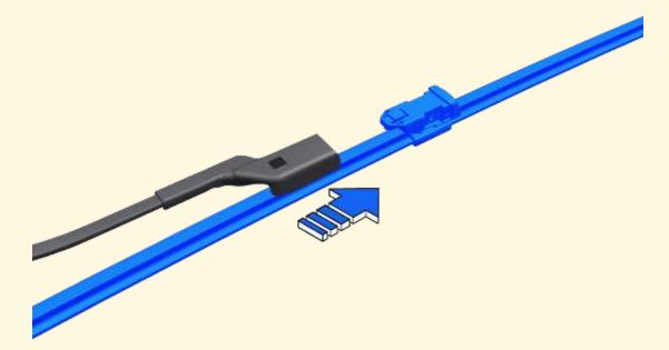
6. Pull the wiper blade in the direction of the arrow to remove it from the wiper arm assembly.
