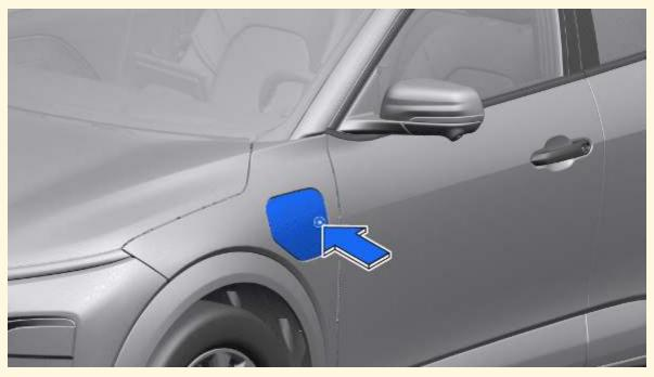
• Close the charge port door and press in the location shown above to lock it.
