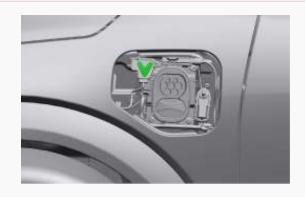
Static green light indicates that the vehicle is fully charged. Pulsing green light indicates that the vehicle is charging.
