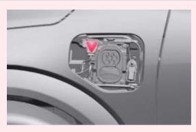
Static red light indicates a faulty connection or charger contains no charge.
