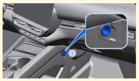
The vehicle is equipped with a power outlet, located on the right side of the Center Console. To access the Low Voltage Outlet, remove the protective cap. The power outlet is suitable for accessories requiring up to a maximum of 12V / 120W.
