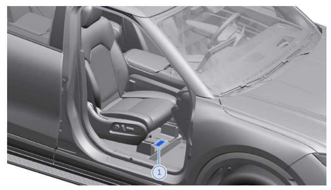
• On the cross-member under the passenger seat. To view lift the carpet flap
