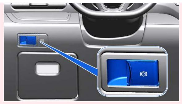
To disengage Electronic Parking Brake (EPB) depress the brake pedal and push the EPB switch.
