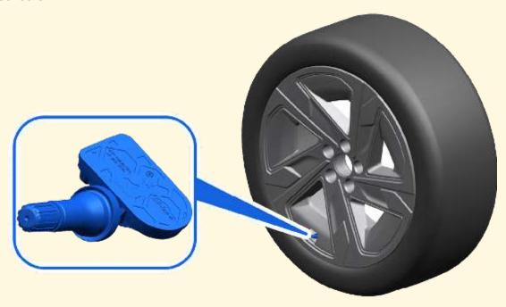
The TPMS system uses sensors in each tire that transmit real-time information on tire pressure and temperature. The sensors are attached to the valve.
