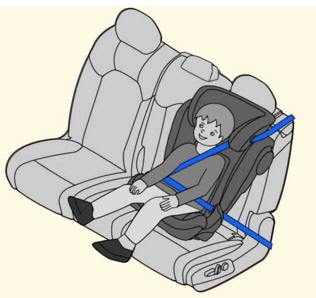
A booster seat child restraint system is used when a child exceeds the height or weight limit of a forward-facing child restraint system. Booster seats are designed to work in conjunction with the vehicle's existing seat belt system. A booster seat positions a child's body to ensure correct routing of a seat belt across the shoulder and lap areas, avoiding contact with the face, neck, and stomach.
